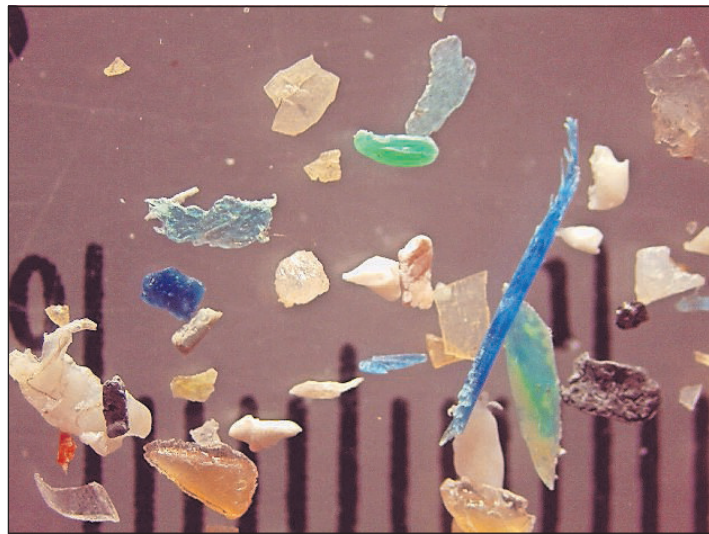
This is a contributed photo of microplastics (shown here with a one-inch ruler behind them), which are pieces of plastic smaller than 5 millimeters wide. They were found in water samples taken from Great Lakes tributaries. A SUNY Fredonia professor involved in the study says microplastics are in lakes, rivers and creeks everywhere, including Erie County. CONTRIBUTED PHOTO
