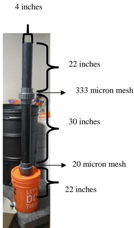
Figure 5.2. Filtration column with height specifications
